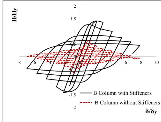
Figure 5. Effect of longitudinal stiffeners.
